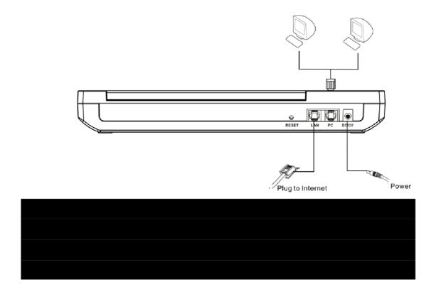
Connect the network cable linking the network to the LAN port, and the configuration PC or other shared PC in the network to the PC port. The LAN port can be connected to the ADSL Modem, Switch or Ethernet private lines. The SMB32 supports fixed IP and IP acquisition through DHCP and PPPoE.
