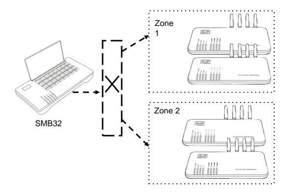
When schedule mode is used (schedule mode = schedule), devices of different zones will automatically exchange their SIM cards when it is time for schedule, so as to realize the automatic roaming of SIM cards. When this configuration is used, chaos mode is adopted for the relationship between the SIM cards and the remote-end devices.
